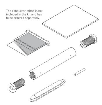
The kits CS-150-xx-PI are designed to connect a PI cold lead cable to a polymer insulated (PI) series heating cable as well as to splice two PI heating cables. The kit employs a two component silicone compound to provide durable and flexible moisture proof encapsulation.
